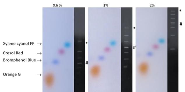
**Figure 2:** Dependency of gel % on dye front position. The four Ampliqon Loading Buffers were run for 75 minutes on either 0.6 %, 1 % or 2 % agarose gel along with a DNA marker. The gel was pictured on white light and UV light and the dyes were correlated to the marker. \*=3000 bp and # = 700 bp.
