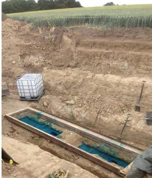
**FIGURE 74.** BB8 dye tracer experiment in 3.5 m depth in E3. The infiltration field had to be separated in two because fractures were accidentally disturbed by the excavator in the middle section.
