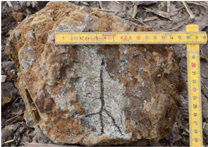
**FIGURE 13.** Soil lump PP2-1 of about 10 kg dug out from excavation E2 at 2.8 m depth. The grey colour is pseudogley covering an exposed fracture with clear casts of  $\approx 0.5$  mm wide, and broad, 3 mm wide, root biopores with organo-mineral fillings.
