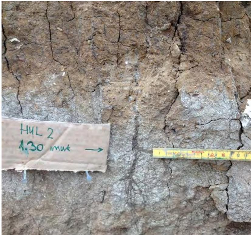
**FIGURE 24.** Transition from open brown fractures in the soil to grey fractures in the subsoil environment (high-ground excavation 2). The transition was located immediately below tile drain depth. The grey staining of fractures continued to 2-3.5 m depth.
