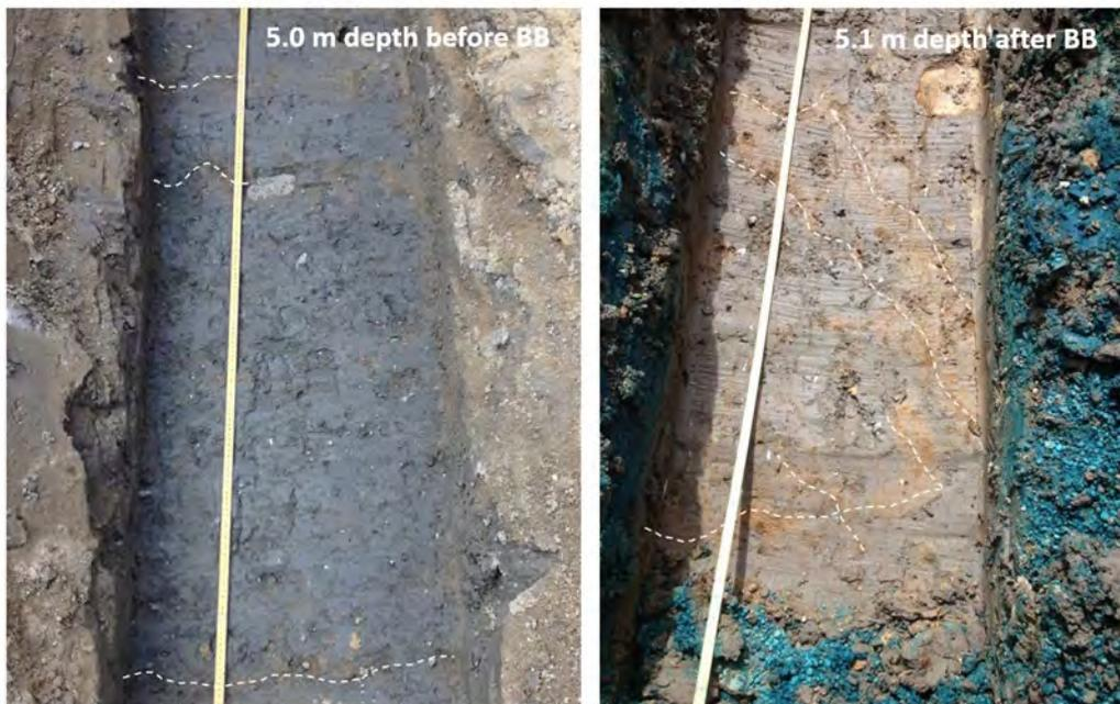
**FIGURE 77.** Surface of BB0 infiltration basin before and after BB infiltration (yard stick 1.2 m long). No BB transport along fractures was observed. Notice increasing oxidation of fractures with depth, indicating upward oxidation of non-visible fractures in the grey clay from oxidizing conditions below (Figure 76).
