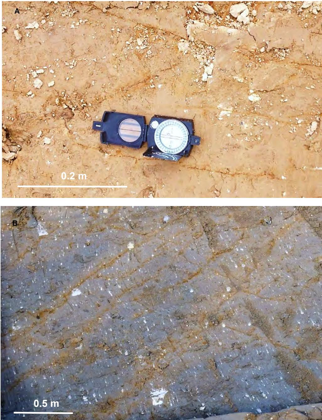
**FIGURE 25.** Appearance of Fe/Mn-oxide stained and infilled tectonic fractures (red fractures) in the high-ground excavations. (A) Red fractures on horizontal surface in yellowish brown oxidized till in 3.5 m depth. (B) Red fractures on horizontal surface in grey reduced till in 5 m depth.
