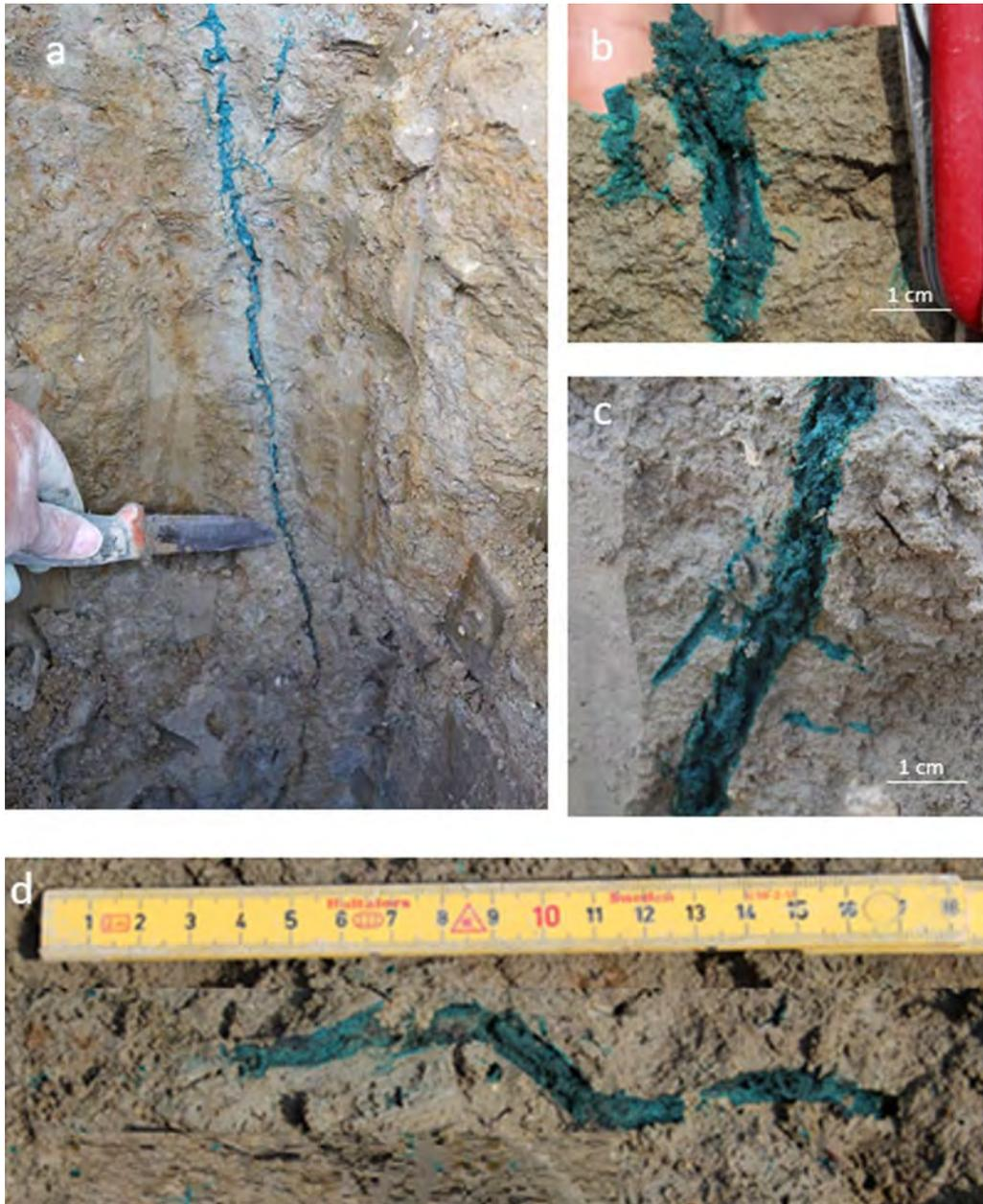
**FIGURE 81.** BB dye tracer migration in fossil roots BB9 infiltration field. (a) Dyed root in 2-2.5 m depth extending from oxidized clay into underlying reduced clay. (b) Dyed root in oxidized clay in 1.5 m depth, and (c) in reduced clay in 2 m depth, (d) Horizontal surface in reduced clay in 2 m depth with dyed root.
