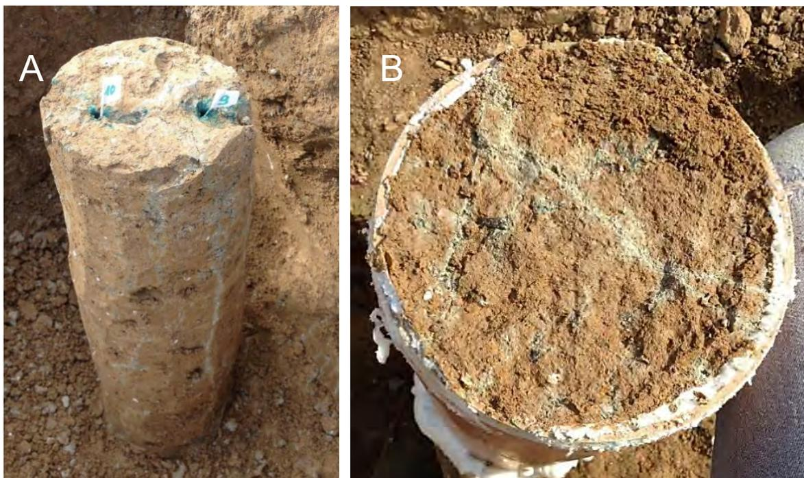
**FIGURE 48.** Sampling of XRT Column 1 from BB1 in 1.1-1.6 m depth (C-horizon) in E2. (A) Side view showing two large worm burrows dyed with infiltrated Brilliant Blue (BB) tracer, and grey fractures penetrating the column vertically. (B) View of bottom of bottom of column showing grey fractures with BB dye tracer migrated along the fractures.
