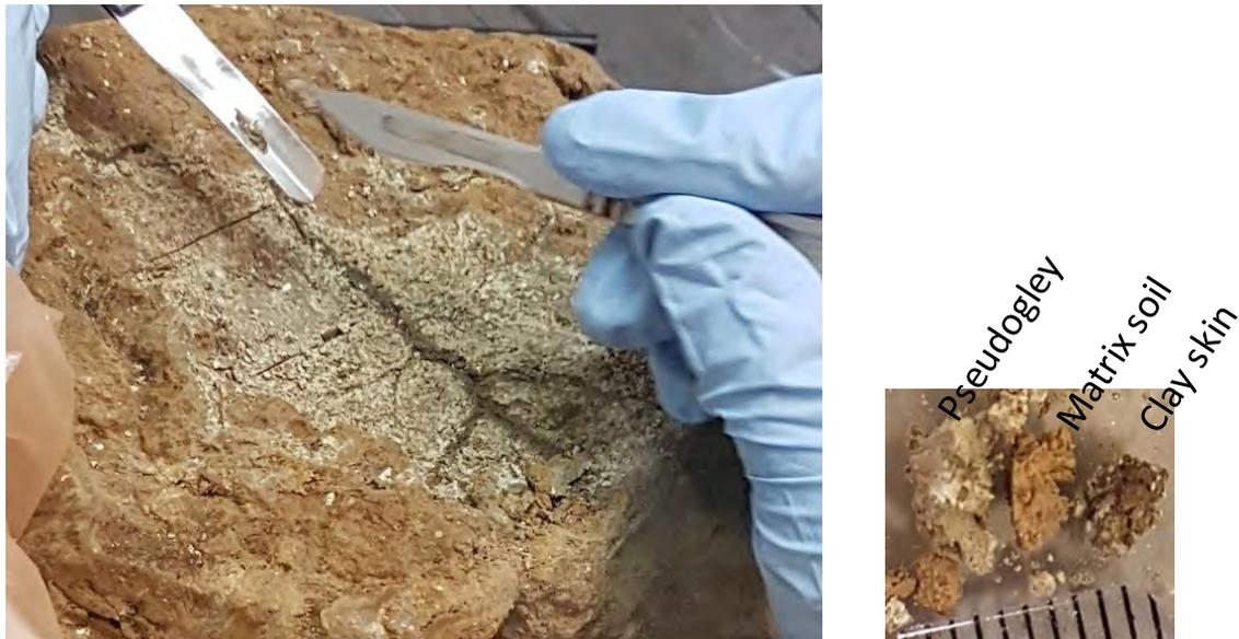
**FIGURE 14.** Sampling of the fracture/biopore lining and fracture surface of PP2-1 and three types of material sampled from the block and fracture.
