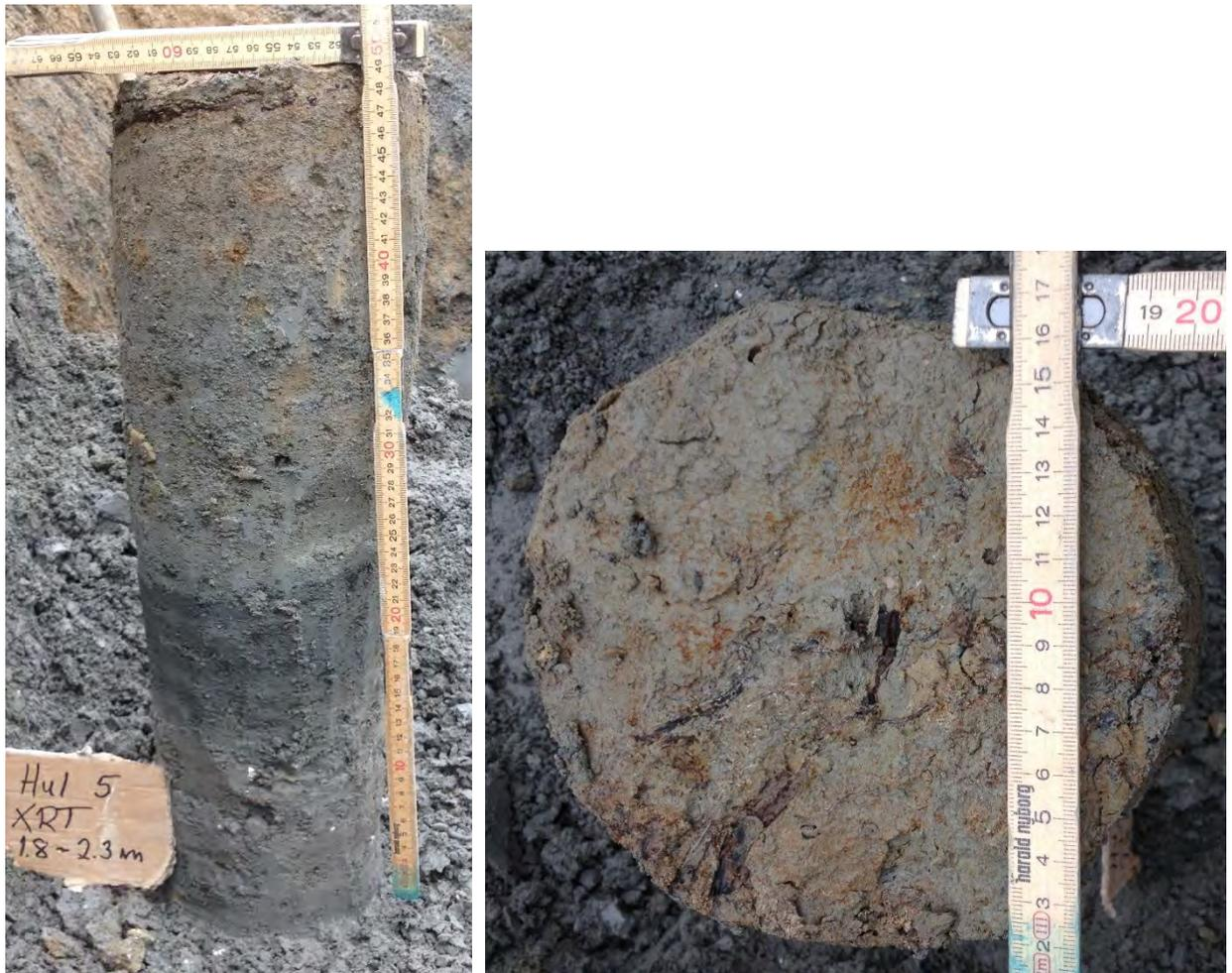
**FIGURE 83.** XRT Column 4 from 1.8-2.3 m depth in E5. (left) Transition from oxidized to reduced till in upper 10-20 cm of column with sub-horizontal fossil roots in top of column. (right) The top of the column shows horizontal and vertical fossil roots from *A. glutinosa* (Red alder) dated 2,984 -2,880 Cal BP.
