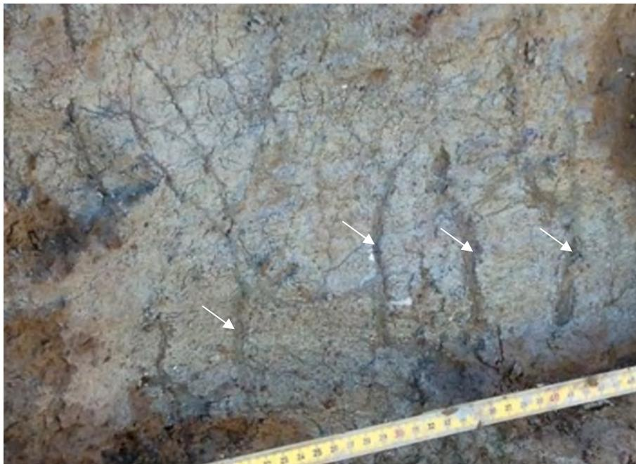
**FIGURE 43.** Large root casts (arrows) inside grey fracture at 2.8-3 m depth in E2 (high-ground). The root casts are flattened inside the fracture, which suggests that the size of the original roots resembled the tree roots found in the low-ground excavations (Figure 38 to Figure 41).
