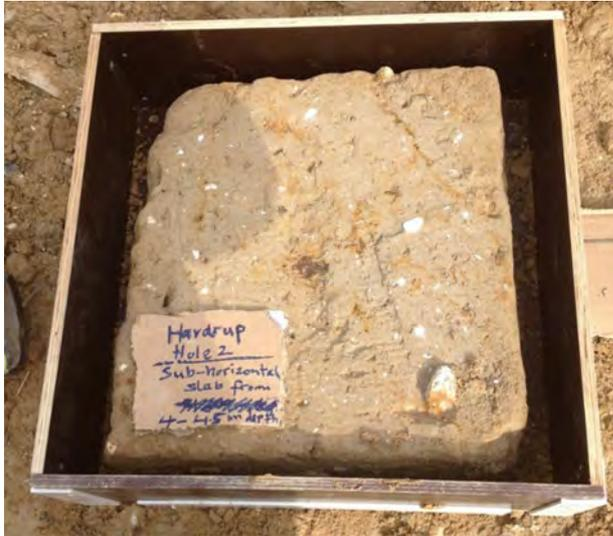
**FIGURE 69.** Intact block containing red fractures in oxidized till collected from 4-4.5 m depth in E2 for XRT analyses.
