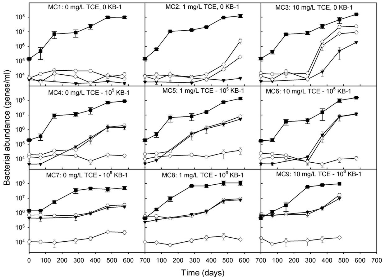
**Fig. 2.** Microbial abundance of specific *Dehalococcoides* spp 16S rRNA genes (○), *vcrA* (▼) and *bvcA* genes (□), and general 16S rRNA genes (■) in the nine microcosms (MC), with error bars indicating the standard error between three replicate microcosms.
