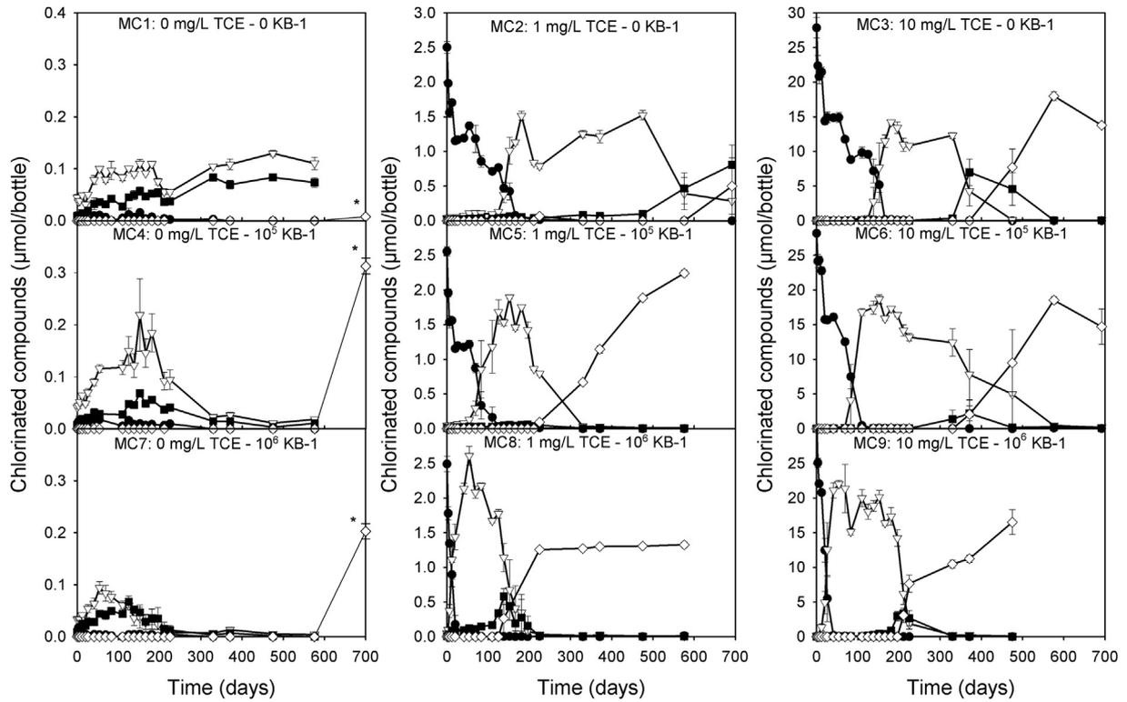
**Fig. 1.** Measured amount of chlorinated ethenes in the nine microcosms (MC), with error bars indicating the standard error between three replicate microcosms (● TCE, ▽ *cis*-DCE, ■ VC, □ ethene). \* These data points were measured with GC-FID after the experiment was ended and can only be regarded semi-quantitative.
